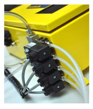
**UVT254 Online** is designed for continuous monitoring of multiple water sources or boreholes in drinking water supply – and to **automatically Exclude and Discharge** what does not meet your high requirements.
